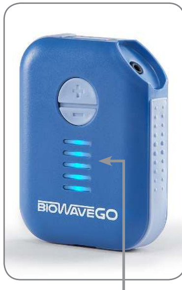
LED Bar Graph Indicator Displaying Signal Intensity
