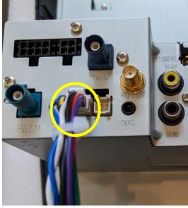
5. The Dynavin camera harness plugs into the back of the unit as pictured in the image to the left (circled in yellow).
