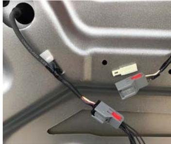
6. Run the Shielded RCA and Power cables to the front of the car behind the head unit.
