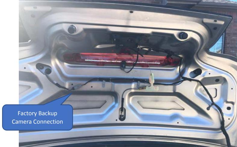
2. 2011 to 2014 cars without NAV use a display screen built into the factory rear view mirror. In order to connect the factory camera to the N7 unit you will need to run your own shielded RCA cable and a +/- set of 12v power wires.
