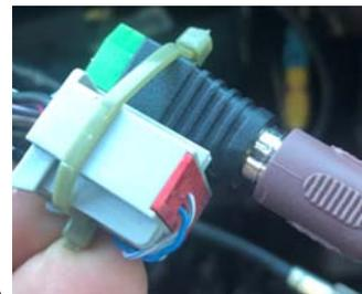
4. Once you have the RCA connection on the factory wiring harness you can plug it into the backup camera harness provided with the N7 unit. You only need to connect the RCA/Video connection. The factory camera will continue to get it's 12v power from the factory wiring harness.
