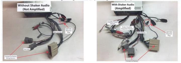
Cars with factory amplifiers <u>may</u> require the use of the included amplifier retention harness. This will provide a lower-level output from the Dynavin/Navos to match the factory amp. Not all cars will require this harness. It takes trial and error to determine what works best for your car.
