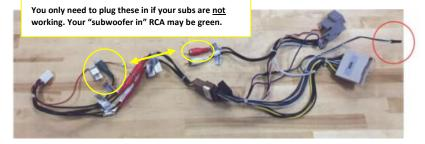
Ensure the red circled 4-pin plug off of the back of the unit (pictured left) is connected and plugged in the <u>correct direction</u> to the 4-pin plug on the main harness "9000". The image below shows the proper orientation in which to plug them in to each other.
