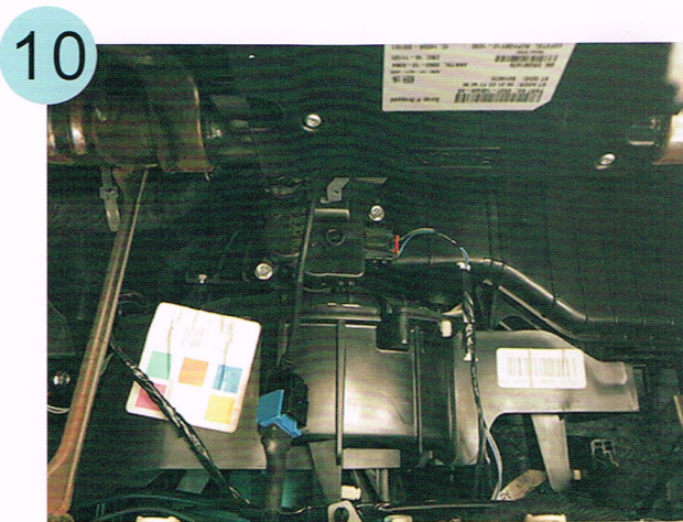
10. Connect Dynavin USB adaptor cable to the factory USB cable
