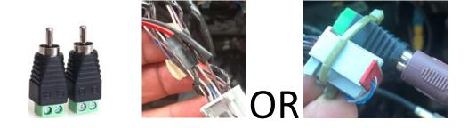
4. Once you have the RCA connection on the factory wiring harness you can plug it into the backup camera harness provided with the N7 unit. You only need to connect the RCA/Video connection. The factory camera will continue to get it's 12v power from the factory wiring harness.
