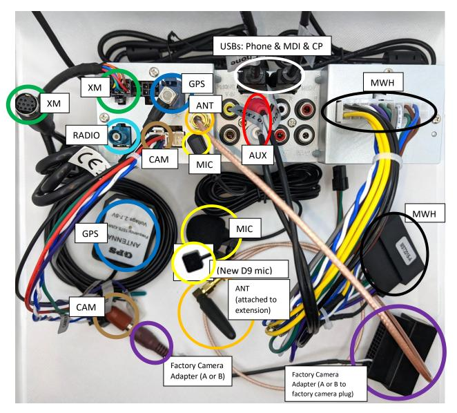
(XM) SiriusXM Adapter Cable: For use only when installing the SiriusXM SXV300 tuner for built-in satellite radio.
