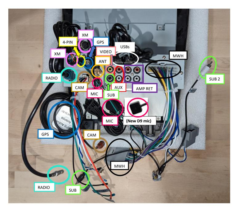
(XM) SiriusXM Adapter Cable: For use only when installing the SiriusXM SXV300 tuner for built-in satellite radio only.
