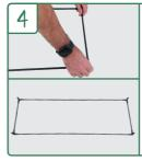
Connect the long poles from Step 3 using two short poles.
