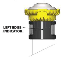
**1.** Align the nozzle to the left most edge of desired coverage area (arc).
