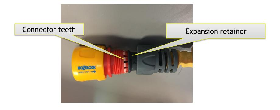
3. Screw nut onto the connector ensuring there's no cross threading and no connector teeth deformed/trapped, continue until it is fully tightened.
