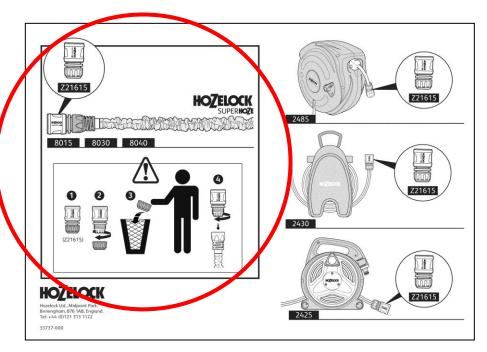
The above instruction leaflet will be sent out with the replacement connector and illustrate that the nut should be discarded when used with Superhoze
