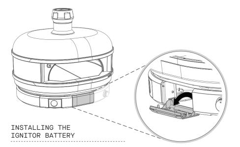
Before using the gas burner for the first time you'll need to install an AAA battery into the ignition module. To do this open the front hatch, the module will be inside and to the left. The module is held in place by a magnet, detach the module and pull it to the front hatch before unnscrewing the cap and placing the battery in (negative end first). Return the module to its original position, close the front hatch and you're ready to connect the gas bottle to the oven.
