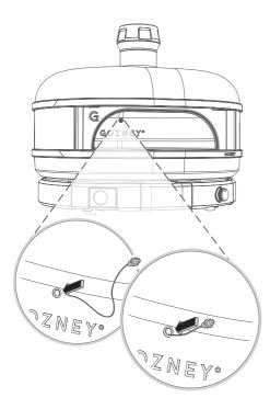
Push the new probe's wires into the hole and feed them through until they are visible from inside the area where the thermometer is normally housed. Hand tighten the probe in place, avoid using a spanner as you may damage the probe.
