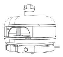
Remove the door and the stone retention wedges before lighting the oven. Do not use the door with gas burner. To light the gas burner press the control knob in and turn the knob 90° until you hear a clicking sound and the burner ignites.
