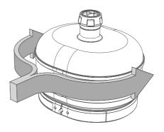
The flue is designed to have a rain guard which has a 1/4 inch gap from the Dome S1.
