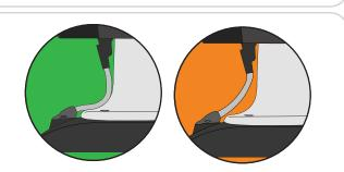
When installing Motor, cable must run against mast (Green). There should not be tension on the cable, or an excessive gap (Orange). If so, move the Motor Pod closer to the system until the gap closes. Cables MUST be taped on to protect the cable.
