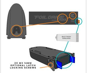
Blue O-Ring MUST be clean, well lubricated & in place. Use Battery Grease to lubricate (Blue Circle).
