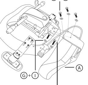
\*The cable of the lumbar goes under the bar of mechanism and back
