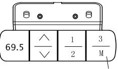
Switch between memory inching/continuous moving
