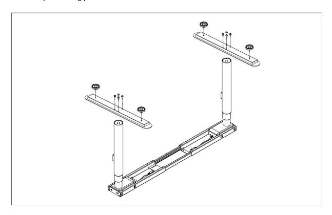
**Step 4**Install the two side brackets with Screws 4 pcs M6x12,
