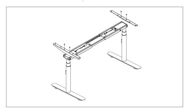
**Step 5**Mount the tabletop and fix it with 14 pcs screws ST4x20; Tighten the screws like D display to fix the top frame. Fix the centre bracket with 2 pcs screws M6x10
