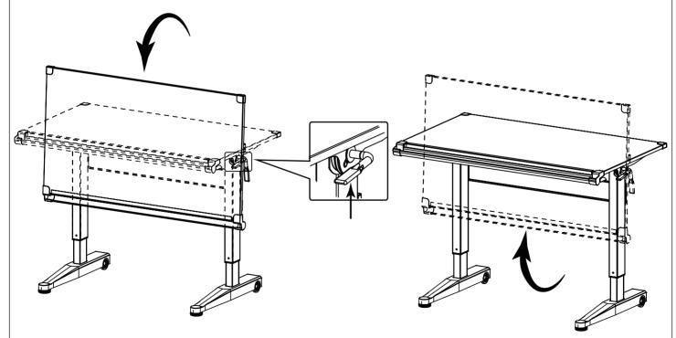
WARNING: The(There is a) danger of falling objects on this table by turning the table up or down, so before turning over, make sure that there are no objects on the table and hold the table with both hands, so children need to be equipped by consultant.
