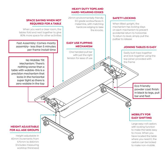
$Standard\ Worktop\ Sizes:\ Frames\ to\ suit\ top\ lengths\ of\ 800-2100mm,\ and\ top\ widths\ of\ 600-750mm$
