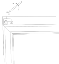
8. Tighten the top hinge pin.
