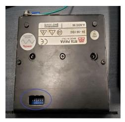
2. Remove the cover on your existing drive and determine if it is set for 400, 800 or 1600 steps using the table below. Set the new drive to the correct configuration for that number of steps.
