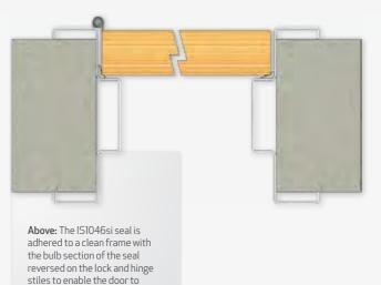
compress against the seal bulb. The seal is fitted to the head of the frame as per the lock stile.
