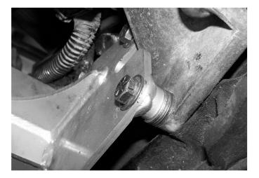
Most Jeep 4.0L models use an alternator bracket that is roughly 5/8" thick. We have found that certain models use a thinner mounting bracket, which changes how our motor mount fits with them. If your Jeep has the thinner (~3/8" thick) alternator mount you will need to shim the forward 2 bolt locations with 3/8" washers as shown.
