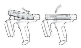
Slide the mobile computer into the Sled until it locks into place. The latches secure the mobile computer to the sled.
