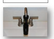
**4.** Attach flush bulb assembly to the sink faucet, slowly turn on water until a thin stream of water begins to flow. Flush for five minutes.
