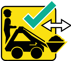
5. TRANSPORT MATERIAL WITH BUCKET DOWN AND LEVEL
