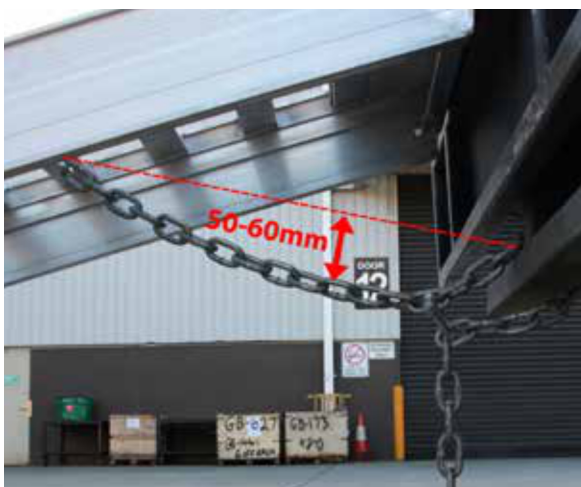
STEP 2 - Ensure the chain between the truck and ramp is not pulled tight. Allow 50-60mm of slack in the chain as indicated on the image above. As the trucks suspension lowers the chain will tighten. Ensure the ramp cannot fall off the back of the truck when the chain is fully extended.
