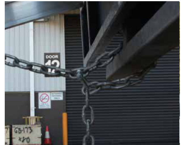
STEP 3 - Lock the chain in place using another shackle. NOTE. Minimum of 8mm closed link chain must be used. The chain must be secured to the vehicle in line with the middle of the ramp.
