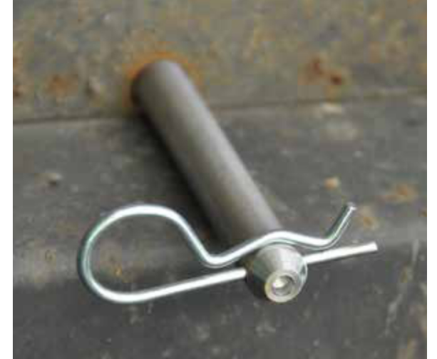
STEP 3 - Secure split pin (R-Clip) to underside of pin.
