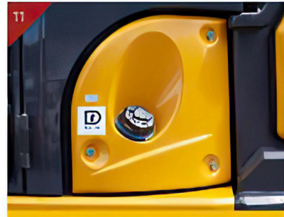
Fuel refill located in a convenient position
