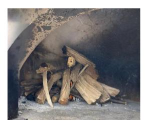
Use fire starter in order to ignite the firewood. After the firewood is completely burned for 3 minutes, move to the air outlet hood of the furnace. Then, add new wood, start the combustion supporting fan, and adjust the fan controller to medium speed (indicator light should be green).
