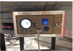
The controller is suitable for DC 5V mobile power supply. The machine can work normally by connecting USB interface and DC 5V mobile power supply. It is recommended to use DC 5V mobile power supply with a capacity of 50000 mA.
