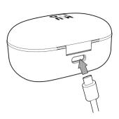
Plug the supplied USB-A to USB-C charging cable into the charging case and a USB-A power supply or certified wall charger. The charging case uses the standard USB voltage. It is not recommended to charge the earbuds using a power supply with a higher voltage.
