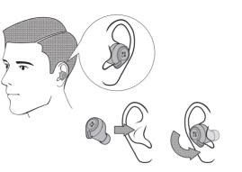
Insert the Earbud into your ear and rotate to fit comfortably. Ensure that the microphones (pointed portions of the earbuds) are pointed towards your mouth for best output.
