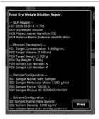
**Step 4**: If no balance is connected, enter the final actual weight of the solution manually. After confirming the weight, a dilution report is generated. The report is saved to the logs and can be printed if required.
