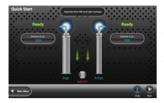
When the Quick Start button is selected from the Main Menu the user will be taken directly to the Run screen. From this screen the user can enter a dispense volume for the left and right syringe, using the Parameter Adjustment button.
