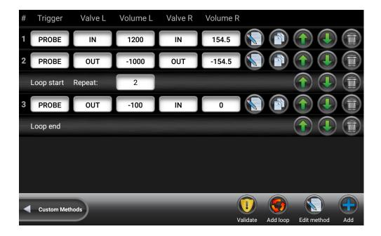
Steps can be moved up and down using the up and bottom arrows in the same line. They can be also duplicated or removed using the corresponding button in the same line.
