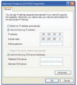
Step 4. Select "Use the following IP address" and enter 192.168.100.50 for the IP address and 255.255.25.0 for the Subnet mask. Press the OK button and close all open dialog boxes so the settings take effect.
