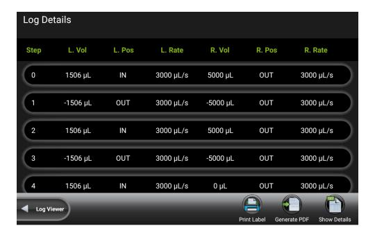
Basic data about each step is assembled into a table with column values as follows:
