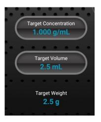
**Step 1:** Enter a target concentration and a target volume. Once the desired concentration of the components and the volume of the standard solution have been entered, the required amount of sample to be weighed is automatically calculated.
