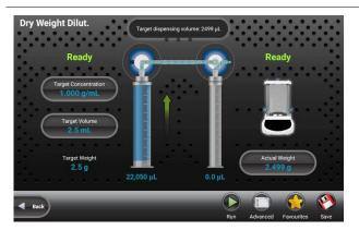
In continuous dispenser mode, both syringes are used to dilute the dry weight.
