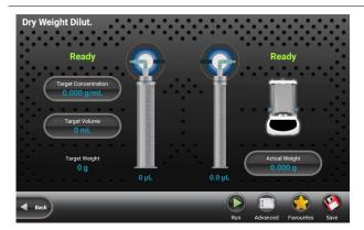
In dual dilutor mode, the Dry Weight Dilution wizard uses the left syringe to aspirate and dispense liquids.
