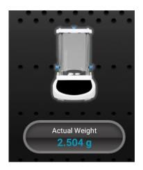
**Step 2:** Weight the dry sample. If the balance is connected via COM1 the actual weight of the sample is displayed automatically. If no balance is connected, enter the actual weight manually.
