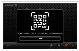
After clicking the quick-access Scan Method icon in the toolbar, a dialog opens awaiting the scan input of the custom method label.
