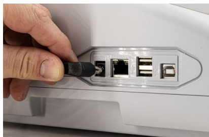
Fig. 2: Connecting the power supply
