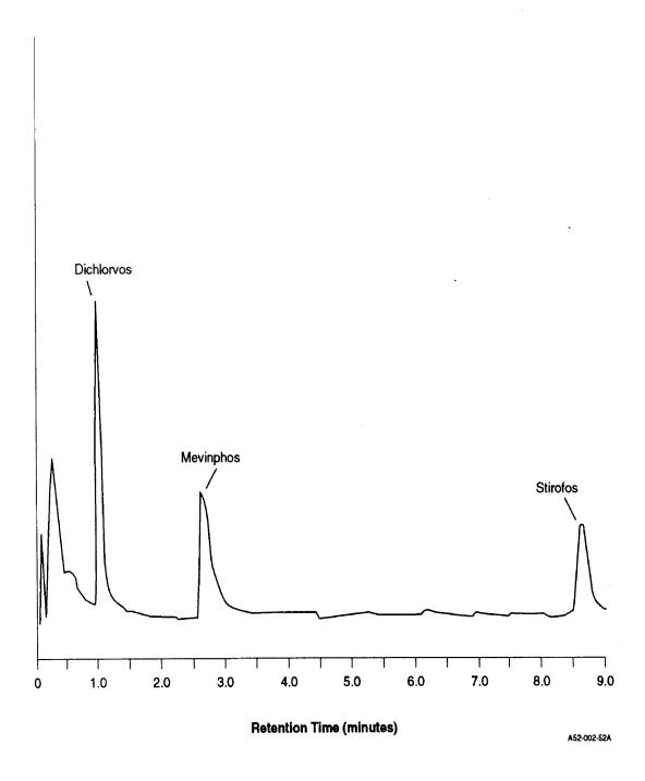
Figure 2. Gas Chromatogram of Organophosphorous Pesticides on Column 1b (for conditions, see Table 1)
