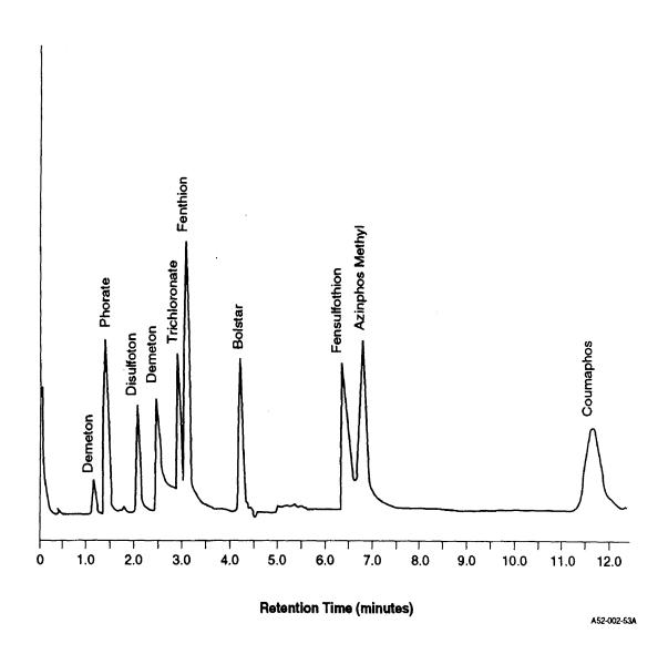
Figure 1. Gas Chromatogram of Organophosphorus Pesticides on Column 1a (for conditions, see Table 1)
