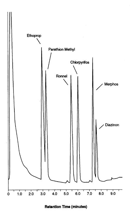
Figure 3. Gas Chromatogram of Organophosphorus Pesticides on Column 2 for conditions, see Table 1)
