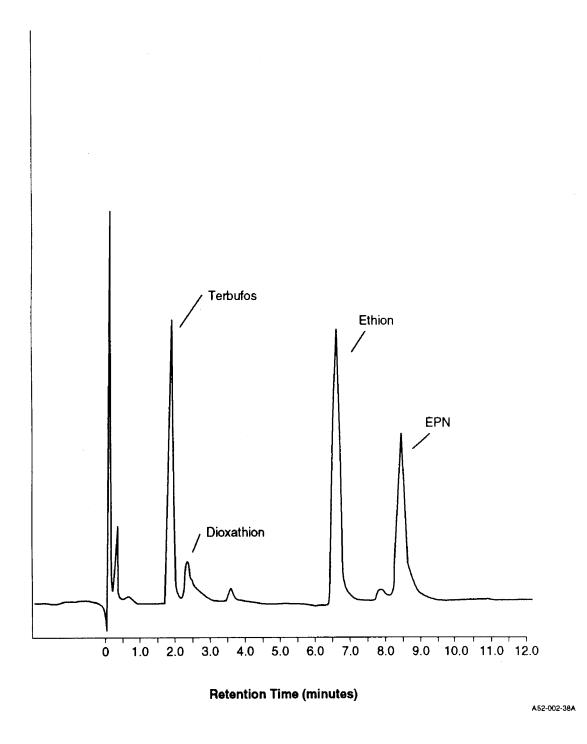
Figure 2. Gas Chromatogram of Organophosphorous Pesticides (Column 2)
