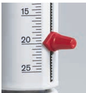
Positive volume setting using interior scalloped track
