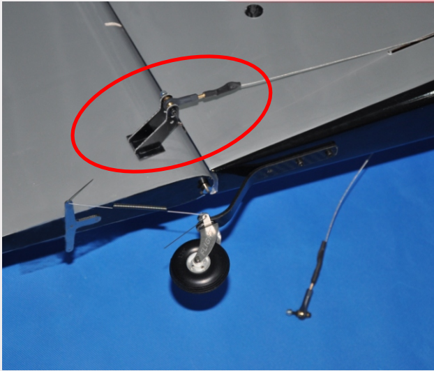
Install rudder servo arms and pushrod.
