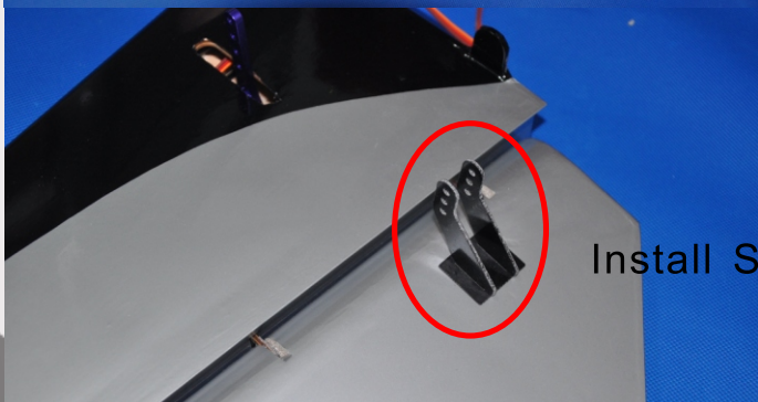
Install stabilizer as photo shown.
