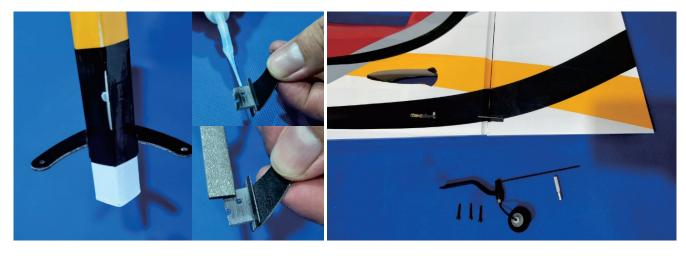
Install the horn of rudder
