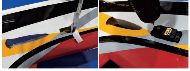
Cut the hole of the elevator
