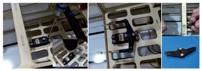
install the servo of the rudder
