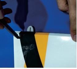
Cut the hole of rudder horn
