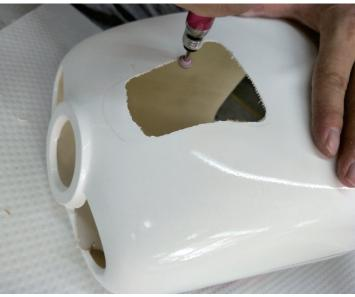
Cut the hole of engine in the cowl
