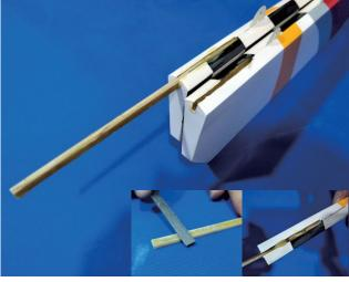
install the servo of elevator
