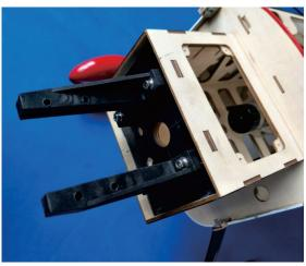
install the Engine bracket
