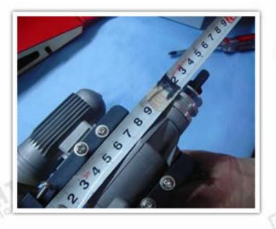
Use the ruler to measure the length from firewall to airscrew, which should be 118 MM.
