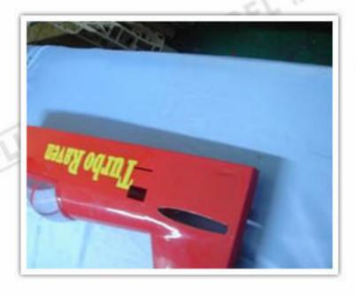
Find out the holes on each sides of the tail fuselage.
