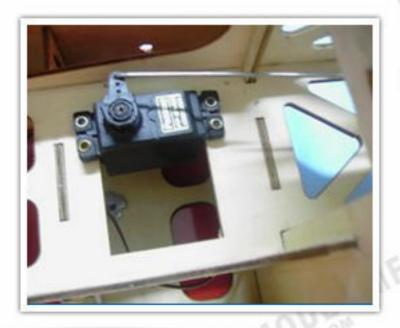
Install the throttle servo and the throttle rod as shown.
