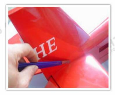
Insert the stabilizer into the prepared hole.
