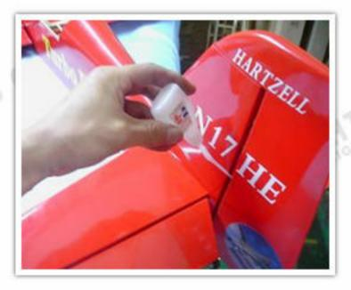
Apply instant type glue to both sides of each hinges of the rudder.
