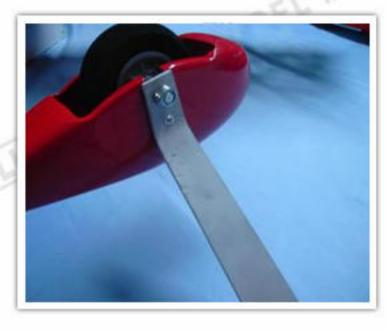
Install the wheel cover, and fix it up to landing gear with TP screw.
