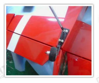
Screw four TP screws to fix up the tail wheel on the tail of the fuselage.
