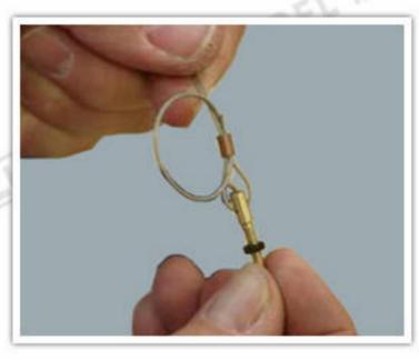
Loop the cable back through the brass swage tube as shown.
