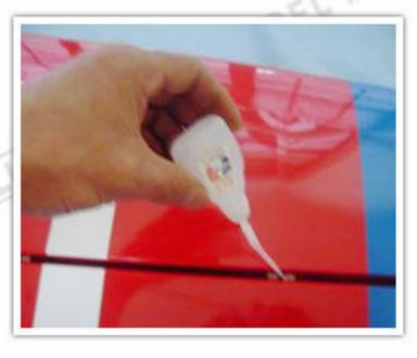
Connect the aileron and the main wing by hinges. Be sure to apply instant type glue to both sides of each hinges.
