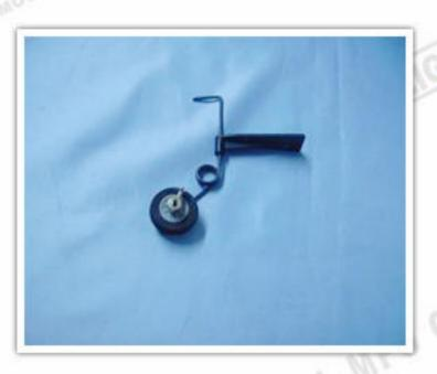
Bent the piano wire as shown.
