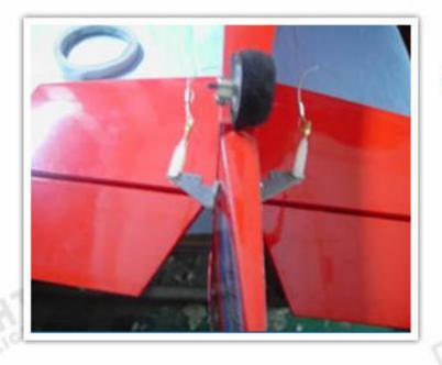
Rudder servo assmble on rudder view. Fixup the tri-horns on both sides of the rudder,then link the collet.
