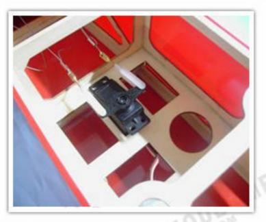
Rudder servo assemble in fuselage view. Fixup the two collets with servo horn as shown.
