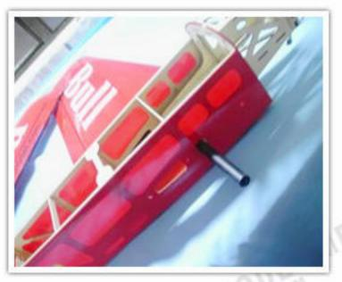
Attach the main wing to the fuselage by bolt.
