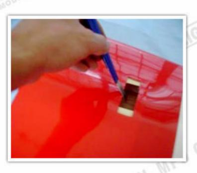
Cut away covering film for the servo on the botom of the main wing ..
