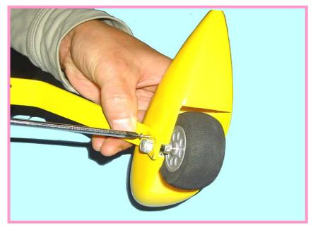
Install the wheel cover, and fix it up to landing gear with TP screw.
