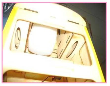
Install the fuel tank into the fuselage, and fixup it with belt.
