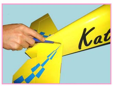
Measure the right position and remove the film from the stabilizer.
