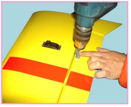
Measure the right position of the tri-horn on the aileron, and drill holes for the screws.
