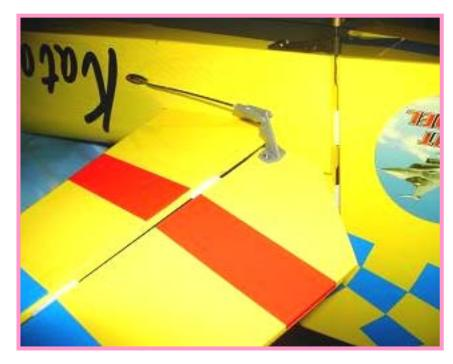
Link the elevator servo to the elevator with pushrod.
