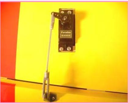
Link the servo and tri-horns with pushrod and straper.
