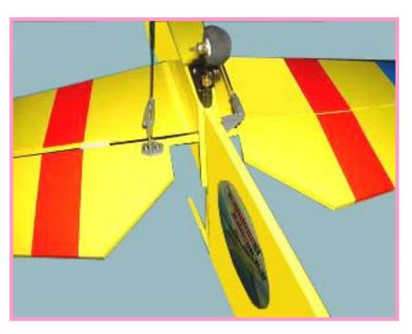
Use the same method to link the rudder servo to rudder.
