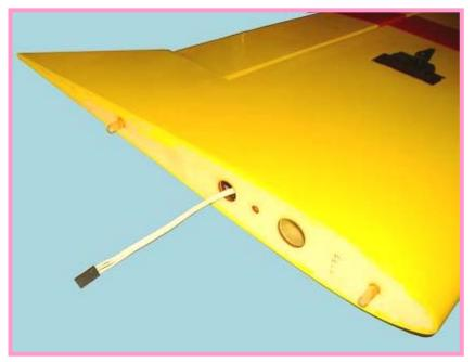
Put the servo into the hole and pull out the servo extension from main wing.
