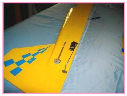
Link the rudder servo to the rudder with pushrod.
