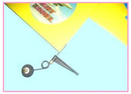
Insert the tail wheel landing gear into the rudder.
