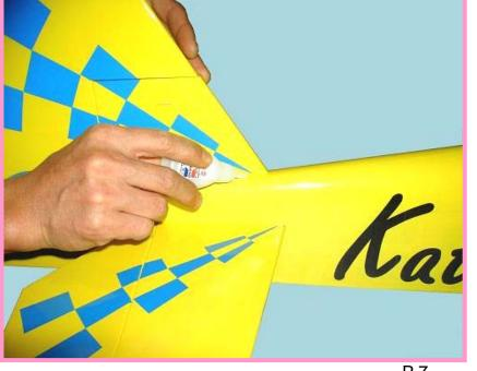
Apply install glue between fuselage and vertical fin.
