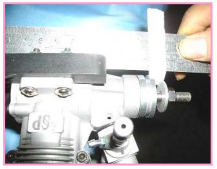
Use the ruler to measure the length from firewall to airscrew, which should be 118 MM.
