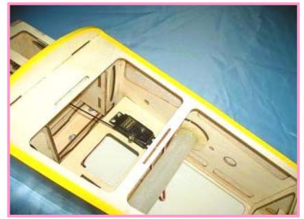
Install the throttle servo and the throttle rod as shown.
