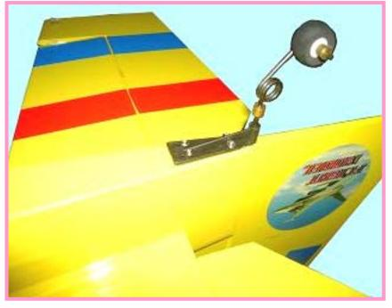
Screw four TP screws to fix up the tail wheel on the tail of the fuselage.
