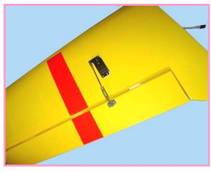
Finished photo for the main wing aileron servo installation.
