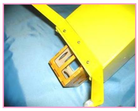
Fixup the landing gear strut to fuselage with 3 bolts.
