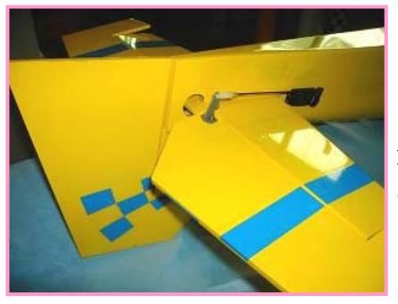
Link the elevator servo to the elevator with pushrod.
