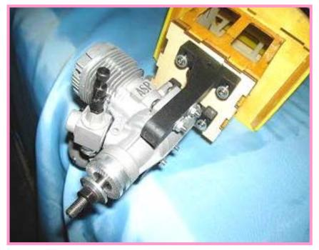
Install the engine mount on both sides with four 3mm screws.
