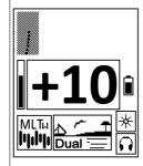
There is a possible case when the graph is in the iron range and the ID number is low and indicates a low-conducting object. It is a low-conductive object masked with soil, ceramics or bricks.
