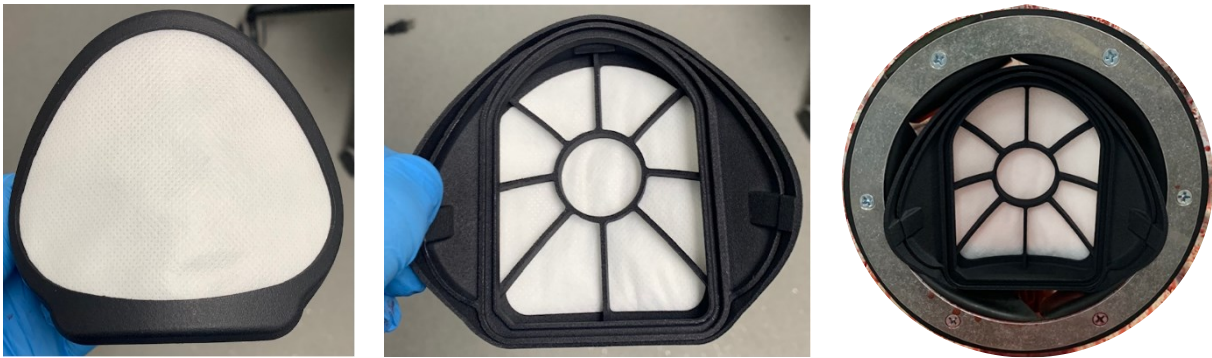
Figure 5.1 front of filter sample in fixture (left), back of filter sample in fixture (middle), fixtured filter sample placed into testing apparatus (right)
