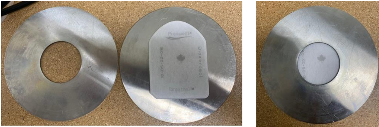
Figure 5.1 Adapter plates with 2-inch diameter holes used to clamp filters for PFE and Breathability Testing
