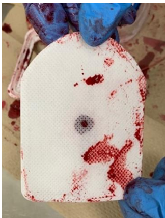
Figure 5.3 the back of a failed blood penetration resistance testing sample showing blood penetration through the back layer
