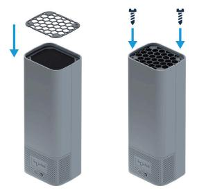
8. Carefully replace the airflow guide. Press down firmly until it clicks into place:
