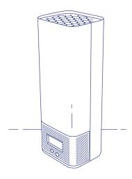
2. Attach the airflow guide by carefully pressing it on to the top of the device and allowing it to click into place:
