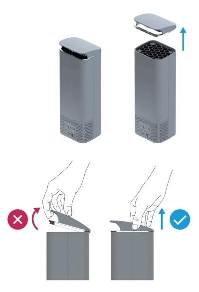
3. Using a Phillips (cross-head) screwdriver, unscrew the two filter grid screws. Remove the top filter grid:
