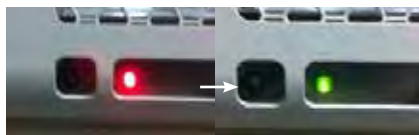
RED flashing GREEN Flashing RED (1 sec) and GREEN (1 sec): Problem with PIRs (one or both)
