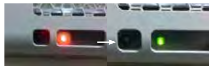
AMBER flashing GREEN Flashing AMBER (1 sec) and GREEN (1 sec): Problem with lamp #1
