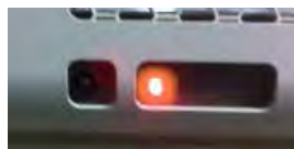
SOLID AMBER Unit is booting (should then switch to GREEN)
