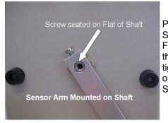
Place the Sensor Arm over the Sensor Arm Shaft End so that the Flat on the Shaft is positioned under the Screw. Using a small screwdriver tighten the Sensor Arm Screw snugly onto the Flat on the Sensor Arm Shaft.
