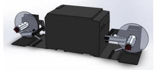
5. Align the Winders with the printer by sliding them forward/backward as necessary until the rear base of the Winders is positioned at the 1.75" mark of the Alignment Plates.
