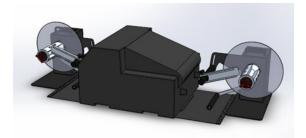
5. Align the Winders with the printer by sliding them forward/backward as necessary until the front base of the Winders is positioned at the 10.5" mark of the Alignment Plates.
