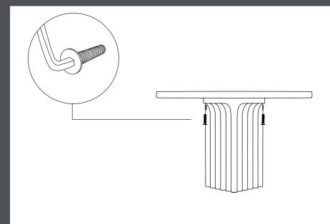
3. Once aligned, insert and align the four screws to secure the installation.
