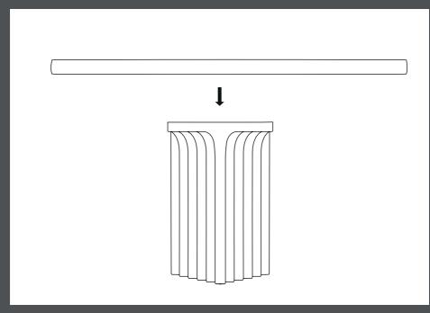
You will need 3-4 people to assist with positioning the tabletop onto the table base. Ensure that the groove on the tabletop aligns with the table base.
