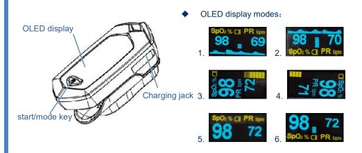
Keys function description: in standby mode, start the key instrument into the working state, pressing this button under working state, can change the display mode.
