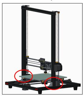
Attention: Put the vertical frame on the chassis, align it with the holes on the aluminum profile of the chassis
