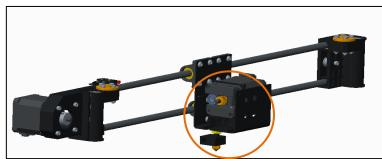
Put the extruder into the L-shaped aluminum holder and tighten the nut
