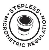
Patented by Eureka, a micrometric system with infinite adjustment points, the only one based on the **lower burr** repositioning
